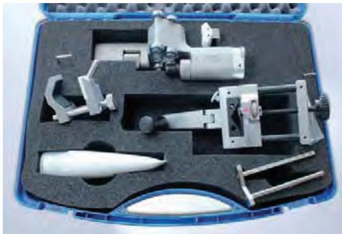
(Figure: Tool case complete, size 1, for cross-sections up to 500 mm<sup>2</sup>)
